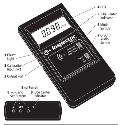
Whenever the Inspector Alert is operating, the red count light (1) flashes each time a count (an ionizing event) is detected.
