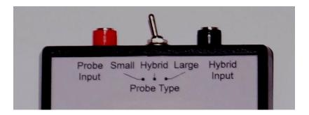
The toggle switch has three positions . To the left is the "small" position for the built in electrode, the tube electrode and the external small flat plate electrode. For the large plate electrode, move the toggle switch to the right to the "large" position. The "Hybrid" centre position of the toggle switch is used with the Fluid probe accessory. For the Fluid probe the black lead goes to the black "Hybrid" connector and the red lead goes to the red "Probe" connector.
