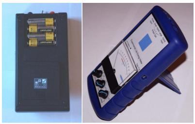
The LM4 comes with 4 "AA" batteries ready to use. When the "low battery" light stays on with a red glow, it is time to replace the batteries. Grasp the rubber boot cover at the bottom of the unit and pull it off towards the back. Once the boot is off, find the battery compartment as shown in the above picture. Slide off the cover, take out the batteries and replace them with a fresh set.
