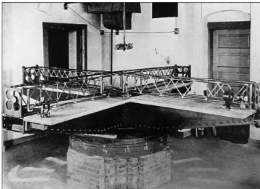
Figure 6. Miller's Control Experiments. A wooden platform has been supplied for the mirrors and optics of the interferometer, inside a building at the Case School.
